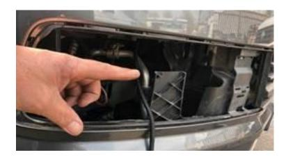
Reconnect the battery. All wiring must be secured to the vehicle, away from any moving or hot parts.
